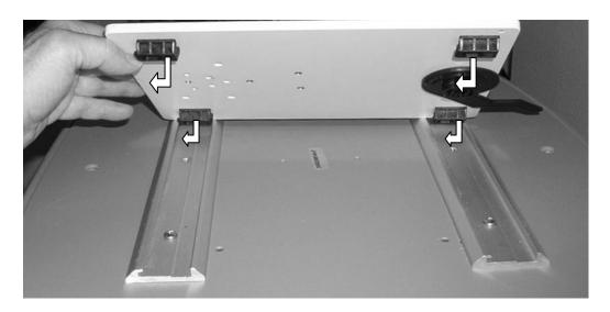
2. Lock the Camlock Plate by moving Camlock Lever from right to left.
