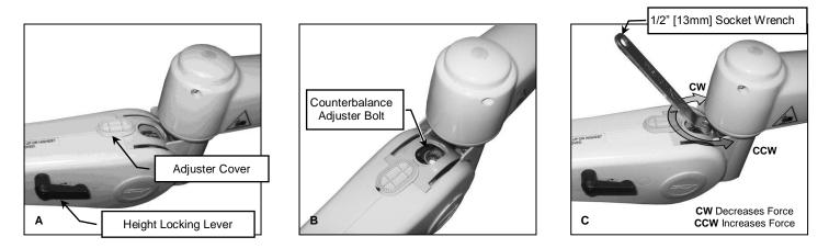
**4.4** Close the Adjuster Cover. Be sure the Adjuster Cover is fully/properly seated and flush to avoid contact with other components on the Arm during movement of the Arm.
