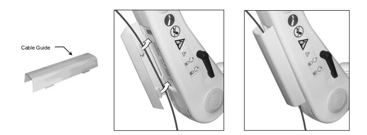
**6.2.** An open cavity beneath the extension with flexible a Cable Cover manages cables going between the channel and rear of the VHM arm. To install cables, push cables into cavity along the center seam of the Cable Cover. Leave some extra cable loose at the front and rear of the Extension to prevent cable binding or damage.
