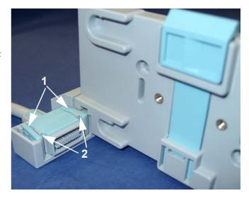
4. Align the feet on the MMS with the locating shoes (1) on the mounting plate and slide the MMS onto the mounting plate.
