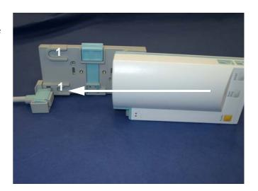
5. Ensure that the cable is securely fixed to the MMS. Once fixed, do not remove the cable from the MMS clamp.
