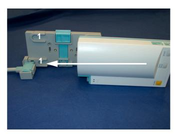
6. Ensure that the cable is securely fixed to the MMS. Once fixed, do not remove the cable from the MMS clamp.
