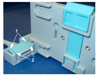
5. Align the feet on the MMS with the locating shoes (1) on the mounting plate and slide the MMS onto the mounting plate.
