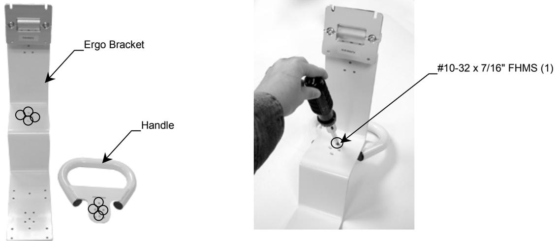
2. Attach the Ergo bracket and Handle assembly to the Roll Stand by aligning the remaining three (3) hole pattern and secure using the supplied #10-32 x 5/8" FHMS (3).
