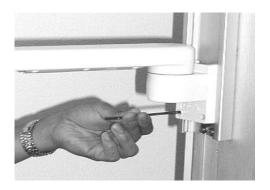
2. Align the screw holes in the Down Post with the threaded holes on the Swivel Fitting. Using the supplied 5/32 (4 mm) hex key and secure the 10-32 x 3/8" SHCS (3).
