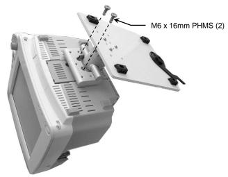
4. Mount monitor/Camlock Mount assembly as described in "Mounting the Camlock Mount" on page 2.
