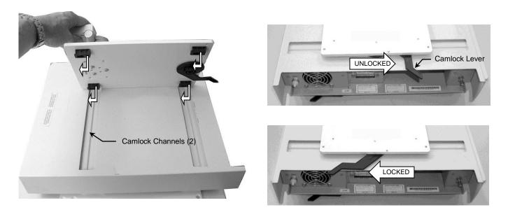
2. To prevent the Camlock Lever from being unlocked, insert one (1) #6-32 x 1/2" PHMS in the threaded hole to the right of the Lever (below). Insert one (1) M4 x 20mm PHMS in each of the two (2) threaded holes at the rear corners of the Mount (below). Stop tightening these screws when they make contact with the bottom of the channel.
