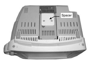
3. Turn Camlock Mount upside down and align Mounting Adapter with corresponding mounting holes in Spacer and monitor. Thread two (2) M6 x 16mm through bottom of Mounting Adapter and into mounting holes in bottom of monitor, ensuring that the Spacer remains between Mounting Adapter and monitor. Adjust tilt tension as necessary. See "Tilt and Swivel Tension Adjustments" on page 4.
