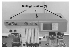
2. Loosen the socket set screws (2 each side) to release the top of the machine. Lift up on the top of the machine and drill in the locations marked in step #1. Use a 1/4" diameter drill bit. Be careful not to drill too deeply, as damage to internal components of the machine could result. Remove all drilling chips.
