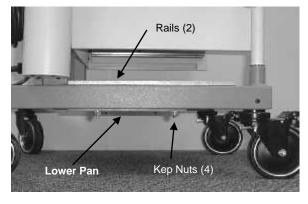
3. Insert the (2) weight bars into the lower pan. Fix them in place by running the (2)  $5/16-18 \times 2 \cdot 1/2$ " or (2)  $5/16-18 \times 1 \cdot 1/2$ " hex bolts through the fender washers and into the inserts in the lower pan.
