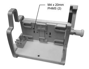
2. Slide the MP2 laterally into the Mount until it clicks into the Dock. Rotate the Latch downward. Press down on the Latch, compressing the foam until the Spring Plunger clicks into position.
