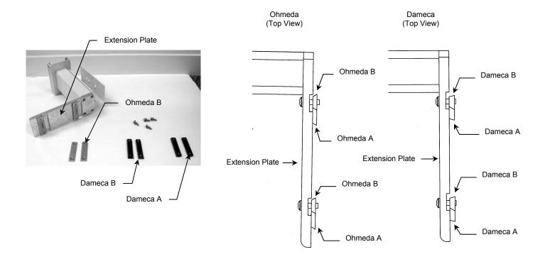
1. Orient Extension as shown and insert the "A Runners" in the dovetail tracks in side support.
