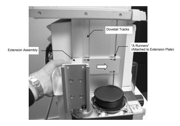
2. Insert "B Runners" in tracks as shown and secure each Runner with two (2) #10-32 x 5/8" PHMS and washers. Position Extension vertically at required mounting position and tighten all screws to secure Extension in tracks.
