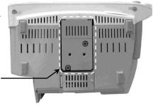
1. Fasten the Philips-supplied Table Mount to the Mounting Adapter with one (1) M6 x 12mm FHMS and two (2) M6 x 8mm FHMS (see below).
