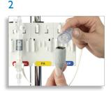
Connect the cable extension of the TRANSPAC<sup>®</sup> 4 transducer to the reusable cable.
