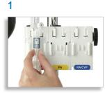
Slide the transducer into the mounting bracket.
