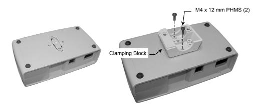
2. Fasten power supply to Post with rear Clamping Block and two (2) #10-32 x 9/16" PHMS as shown below.
