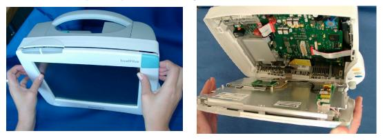
**Reassembly Note:** Make sure the metal sheet on the back of the display is inserted into the noses of the monitor rear housing when reassembling the two halves.
