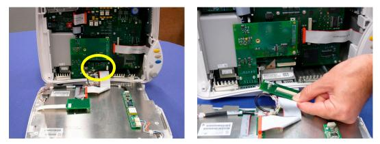
New Sharp/ELO Version - Remove Panel Adapter Board
