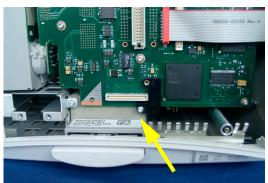
Black Spacer is attached to main board with one screw
