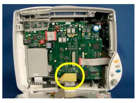
Old LG-Philips/3M Version - Remove Flex Panel Adapter Cable
