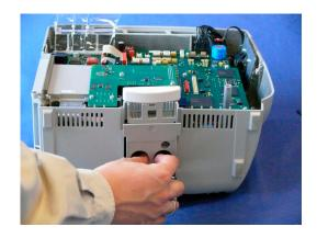
8 Insert the fix mount with the withe release knob cover and secure it with two screws.
