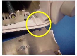
5 Depending on the version of your monitor, unscrew the screws holding the flex panel adapter cable and pull off the flex cable carefully towards you **or** unscrew the panel adapter board and disconnect the board..
