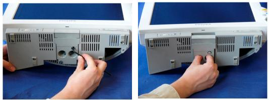
2 The fix mount is delivered with a white release knob cover. Remove this cover and replace it with the grey cover from your fix mount kit.
