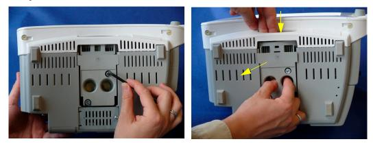
3 Insert the Fix Mount with the white release knob cover and secure it with two screws.
