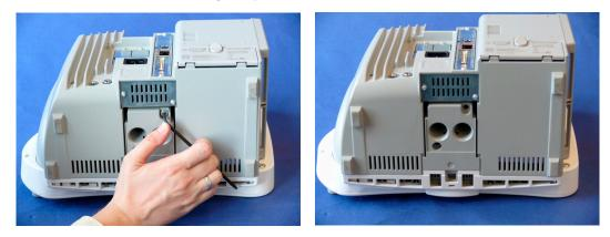
2 Remove the battery from the battery compartment.
