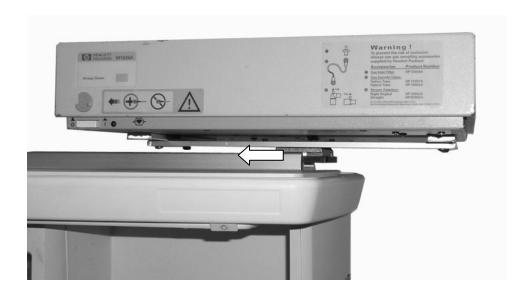
2. Tighten two (2) set screws in the Slide to prevent the AGM from moving in the channel (below). If the Crossbar was rotated (page 2), these screws will be accessed from the front of the AGM.
