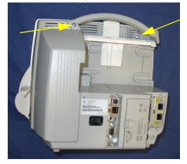
2 Using the same screws secure the bedhanger to the monitor.
