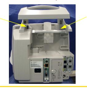
**CAUTION** Make sure the bedhanger is tightly secured to the monitor (1.3 Nm torque) before hanging the monitor on a bed. Loose screws may result in the monitor separating from the bedhanger and falling down.
