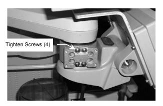
3. Locate four mounting holes in Slide Plate shown below left. Fasten Drop Plate to Slide Plate with four (4) #10-32 x 3/4" PHMS as shown below right.
