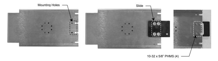
2. Turn Counterweight Cover upside down and slide the Weight Bar into Cover as shown below. Place the Mounting Bracket over the Weight Bar (Bracket fits between Cover and Weight Bar) and fasten Cover to Bracket with four (4) #10-32 x 1/4" FHMS.
