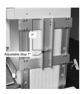
3. Insert Slide (rear of CPU Mounting Pan) in Channel and carefully guide CPU to rest against Adjustable Stop.
