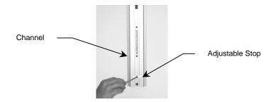
2. Guide Arm Extension into Channel as shown.
