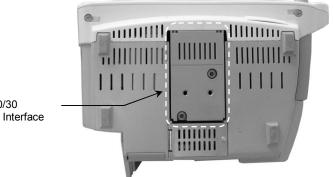
Do Not Attach Table Top Mount if MP20/30 Monitor is Equipped with This Mounting Interface
