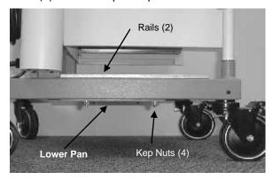
3. Insert the (2) weight bars into the lower pan. Fix them in place by running the (2)  $5/16-18 \times 2 \times 1/2$ " or (2)  $5/16-18 \times 1 \times 1/2$ " hex bolts through the fender washers and into the inserts in the lower pan.
