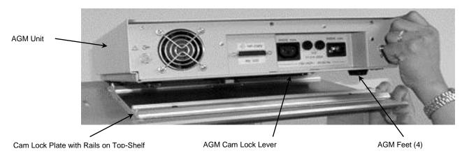
2. Secure the AGM to the Top-Shelf Plate by moving the AGM Cam Lock Lever as shown.
