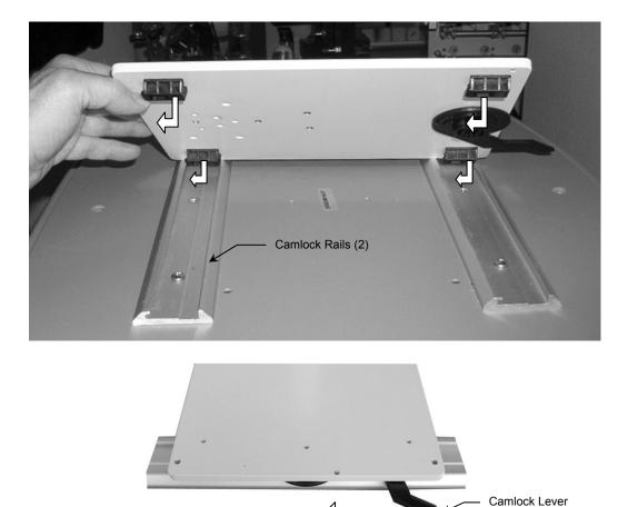
2. To prevent the Camlock Lever from being unlocked, insert one (1) #6-32 x 3/8" PHMS in the threaded hole to the right of the Lever (below right). To further secure the Camlock Mount in the Rails, insert one (1) M4 x 20mm PHMS in each of the two (2) threaded holes at the rear corners of the Mount (below right). Stop tightening these screws when they make contact with the bottom of the Rail.
