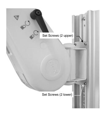
4. Mount the monitor in accordance with Philips Table Top Mount instructions. Attach Down Post if required (see procedure below) and proceed to "Counterbalance Adjustment" on page 4. **Installation Note:** Counterbalance Adjustment must be performed after monitor and FMS are mounted on the Arm.
