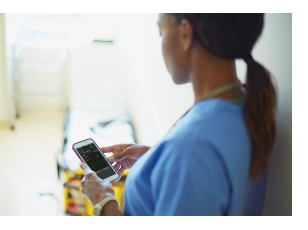
When deployed together with Philips central station and CareEvent, IntelliBridge solutions can deliver alerts from patient care devices — including up to four numerics, four waveforms and associated patient monitoring ringtones - directly to nurses' smartphones. Nurses can determine the validity and priority of the alarm, and make an informed decision to respond, escalate it to a colleague, or rule it non-actionable.
