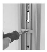
2. While supporting the bottom of the Arm, guide the Slide (rear of Arm) into the top of the wall channel (below left). Slide Arm to desired mounting position and tighten two (2) set screws (bottom of the Slide) with 1/8" hex wrench provided.
