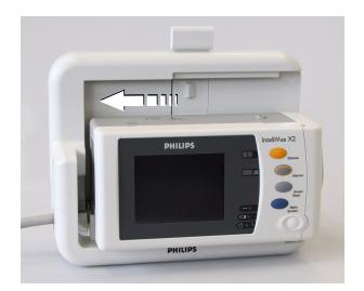
2 You can also combine the MMS, MP2 or X2 with various MMS Extensions, for example the M3015A as shown in the illustration
