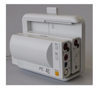
3 To remove the MMS, MP2 or X2 (with or without MMS Extensions) from the Universal Docking Station, release the snap lock (1) and slide out the MMS, MP2 or X2.
