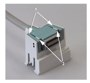
6 Return the cable clamp to its position on the Universal Docking Station.
