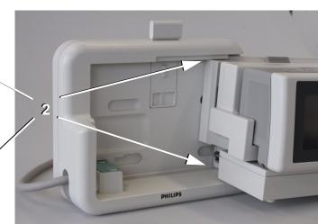
To remove Battery Extension, MP2 or X2, plus MMS Extension combination from the Universal Docking Station, release the snap lock (1) and slide out the Battery Extension.
