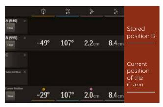
Position Memory stores a previous position and displays it on the monitor above the current position of the C-arm, helping the user quickly return to the desired view with accuracy.
