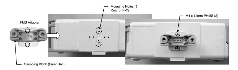
2. Position FMS on Roll Stand Post. Fasten rear half of Clamping Block to front with two (2) #10-32 x 9/16" PHMS (below left). Alternately tighten screws until FMS is secure on post and does not rotate.
