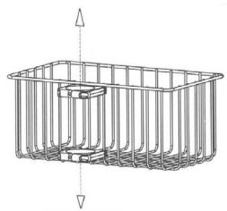
3. Slide the Clips (with Basket attached) over the Roll Stand Post and move the Basket to a position approximately 12" below the top of the Post. Assemble the two (2) #8-32 x 1-1/2" PHMS and hex nuts in the Clips as shown below but do fully tighten the screws at this time. The Basket will be aligned with the Mounting Adapter Assembly later.
