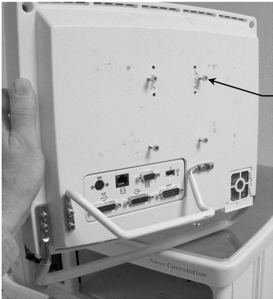
4. Mount ventilator display on Mounting Bracket by hanging the four (4) SHCS in the keyholes. Using the 3mm hex wrench provided, tighten four (4) SHCS.
