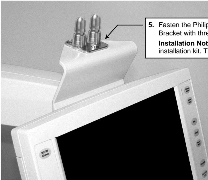
5. Fasten the Philips-supplied table mount to the top of the Mounting Bracket with three (3) M6 x 8 mm FHMS.
