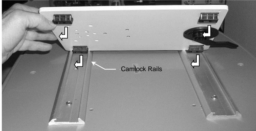
2. Move Camlock Lever from right to left to lock Mount in Rails. To prevent Camlock Lever from being unlocked, insert one (1) #6-32 x 3/8" PHMS in threaded hole to the right of Lever. Insert one (1) M4 x 20mm PHMS in each of the two (2) threaded holes at rear corners of the Mount as shown below. Stop tightening when screws contact bottom of Rail.
