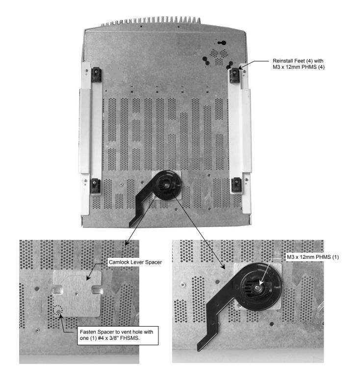
5. Mount CPU in camlock rails according to Philips installation instructions.
