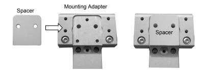
2. Insert two (2) M6 x 16mm PHMS through bottom of Mounting Adapter and thread into mounting holes in bottom of monitor.
